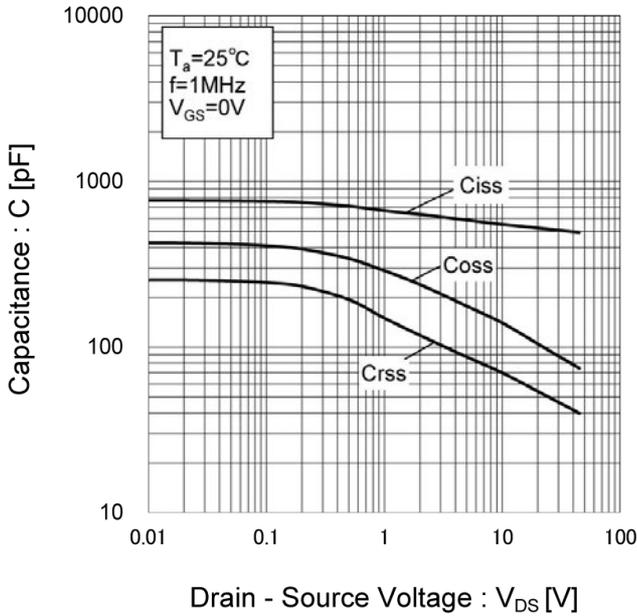
Fig.19 Switching Characteristics
