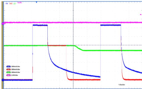
By SW\_SEL command, battery level over  $V_{ODC}$  and below  $V_{ODC}$
