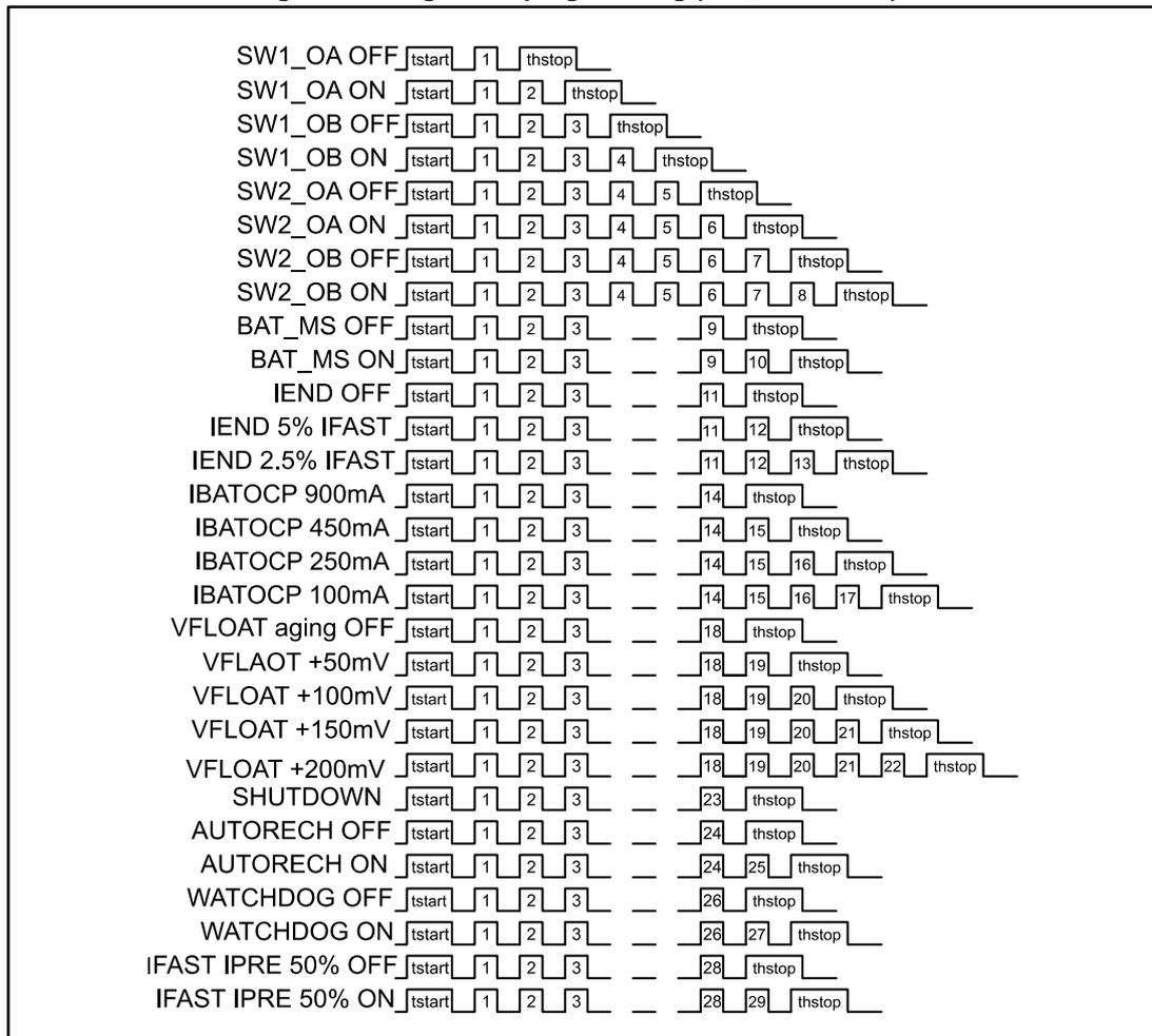
Figure 22: Start and stop timing bit range
