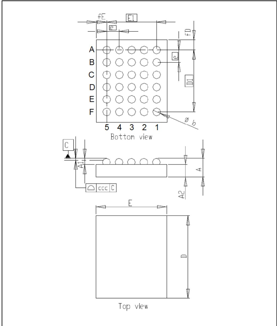
Table 11: Flip Chip 30 (2.59x2.25 mm) package mechanical data
