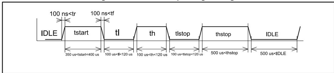
Recommended SWIRE programming pulse width is 100  $\mu\text{s}$  minimum, 120  $\mu\text{s}$  maximum.
