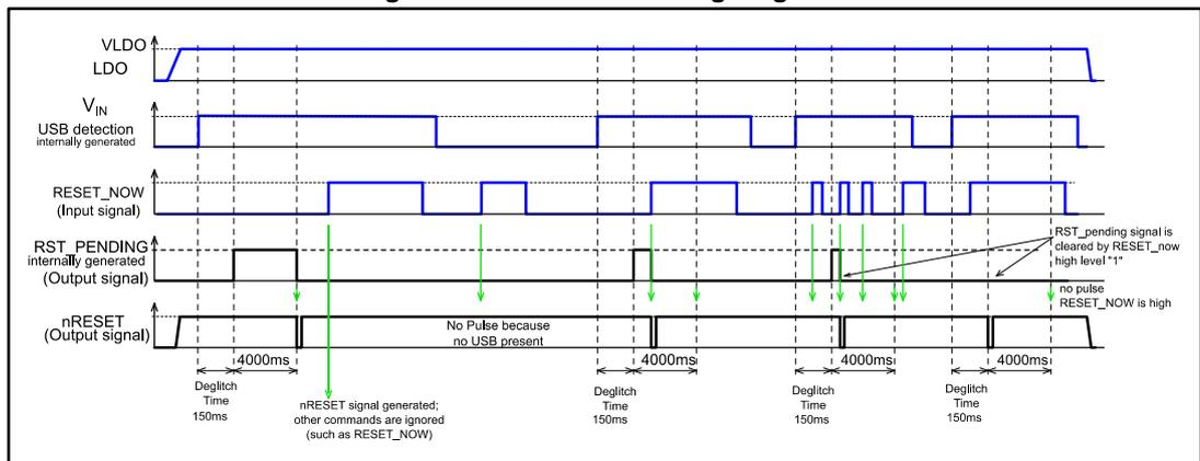
The nRESET pull-up resistor must be connected to LDO pin or to a higher voltage.
