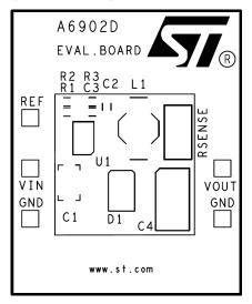
Figure 15. PCB layout (BOTTOM side)
