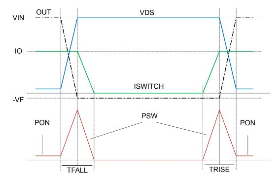
Figure 10. Switching losses
