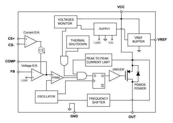
Figure 2. Block diagram
