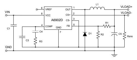
Figure 11. Low-side current sensing implementation
