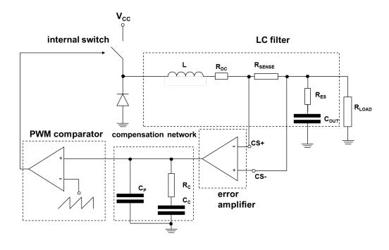
The poles of this transfer function are (assuming  $Cc >> C_0 + C_P$ ):
