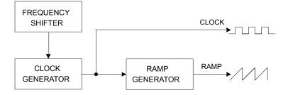
Figure 4. Oscillator circuit block diagram
