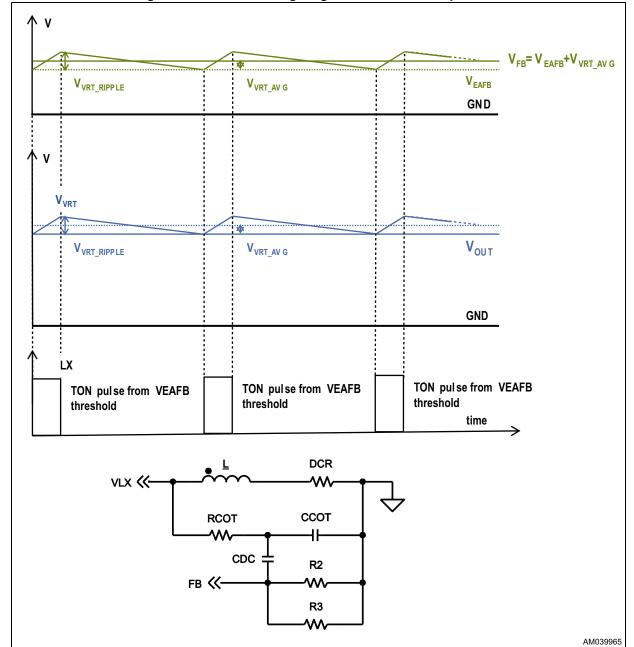
Figure 16. Virtual ESR signal generation in CCM operation
