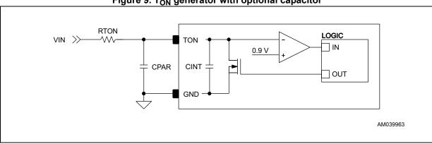
Figure 9. Ton generator with optional capacitor
