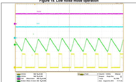
Figure 19. Low noise mode operation
