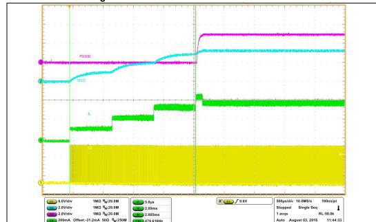
Figure 18. Soft-start feature with resistive load
