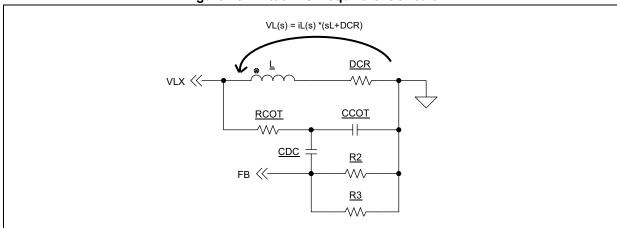
Figure 15. Virtual ESR equivalent circuit
