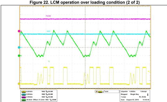
When the load current is higher, the  $I_{\mbox{RIPPLE}}/2$  the regulator works in CCM.
