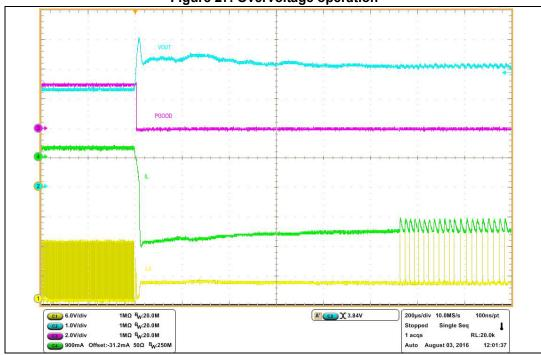
Figure 27. Overvoltage operation
