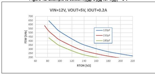
Figure 12. Example to select  $R_{TON}$ ,  $C_{TON}$  for  $V_{OUT} = 5 V$
