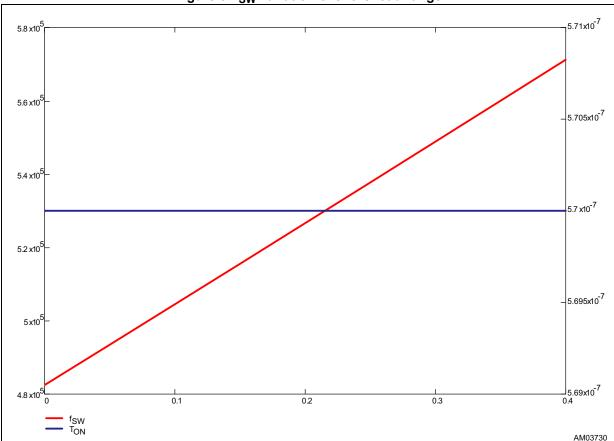
Figure 8. f<sub>SW</sub> variation over the load range
