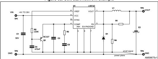
Figure 32. Soft-start network example
