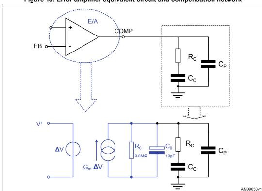
The poles of this transfer function are (if  $C_c >> C_0 + C_P$ ):
