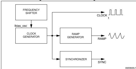
Figure 5. Oscillator circuit block diagram
