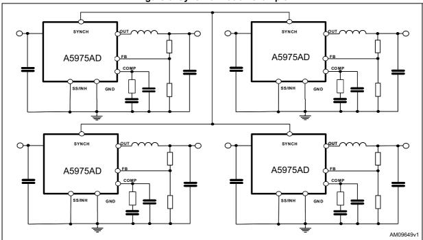
Figure 6. Synchronization example
