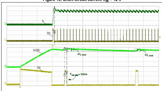
Figure 19. Short-circuit current  $V_{IN}$  = 12 V
