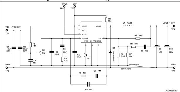
Figure 22. Demonstration board application circuit
