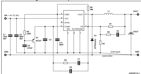
Figure 31. MLCC compensation network circuit
