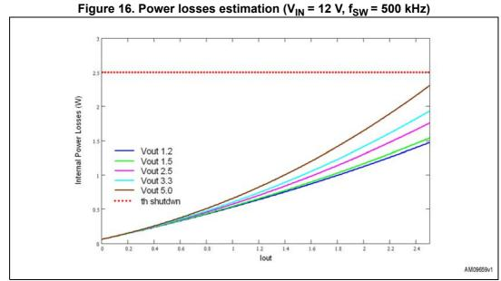
Figure 16 plots the power losses for V<sub>IN</sub>=12 V and the main output rails.
