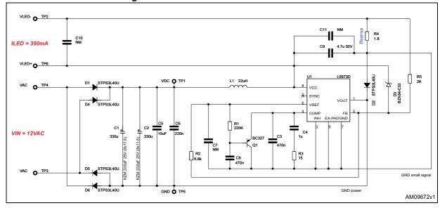
Figure 29. 350 mA LED boost current source
