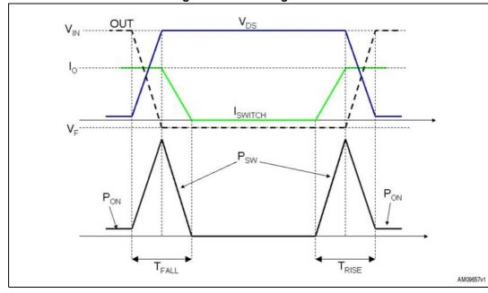
Figure 14. Switching losses
