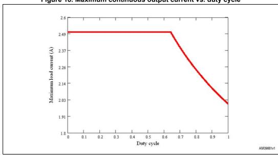
Figure 18. Maximum continuous output current vs. duty cycle
