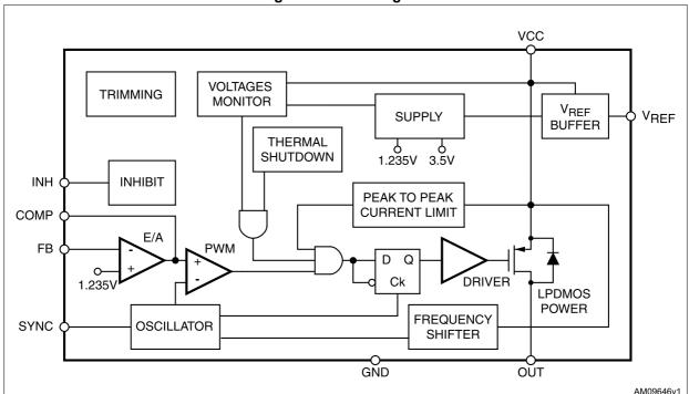
Figure 3. Block diagram
