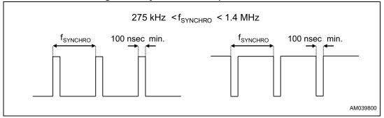
Figure 34. Synchronization pulse definition
