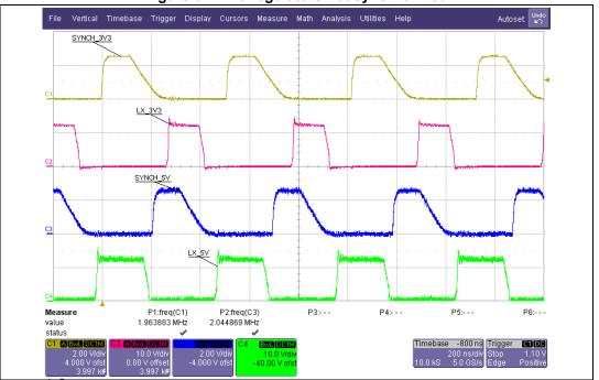
Figure 32. Two regulators not synchronized
