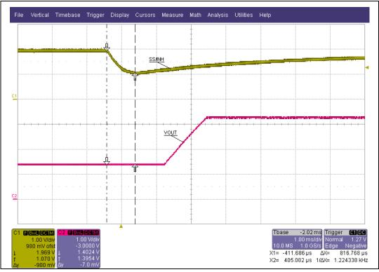
Figure 9. External soft-start after UVLO or thermal shutdown
