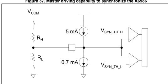
Figure 37. Master driving capability to synchronize the A6986
