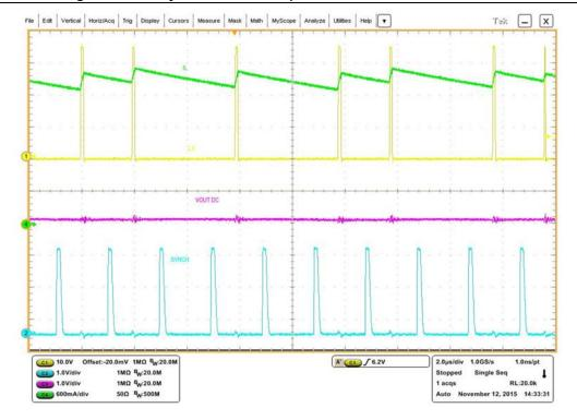
Figure 18. Valley current sense operation in overcurrent condition
