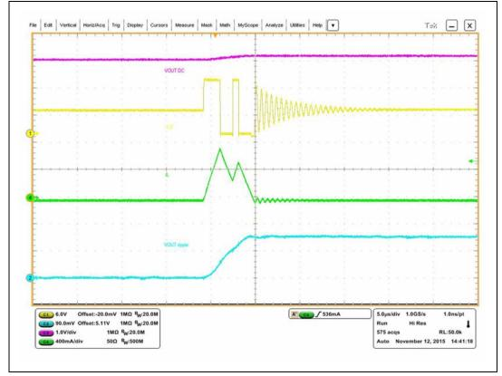
Figure 14. LCM operation at zero load
