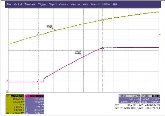
Figure 8. External soft-start network V<sub>STEP</sub> driven
