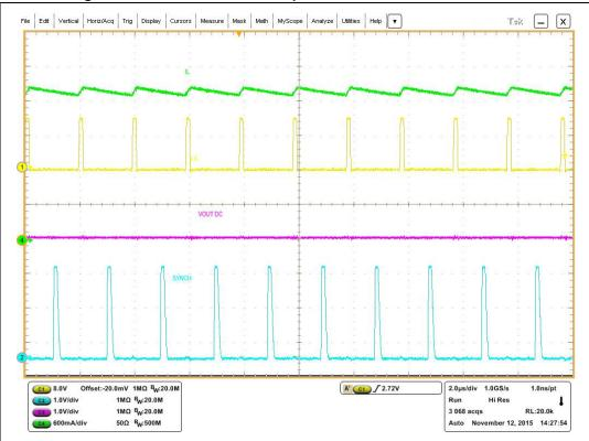
Figure 19. Peak current sense operation in overcurrent condition
