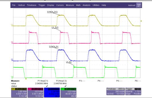
Figure 33. Two regulators synchronized
