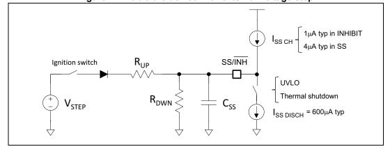
Figure 7. Enable the device with external voltage step
