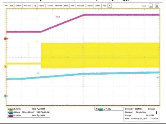
Figure 6. Soft-start phase with precharged COUT
