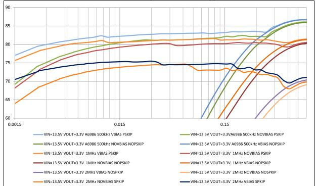
Figure 44. Efficiency curves over  $f_{sw}$ :  $V_{IN}$  = 13.5 V -  $V_{OUT}$  = 3.3 V (log scale)
