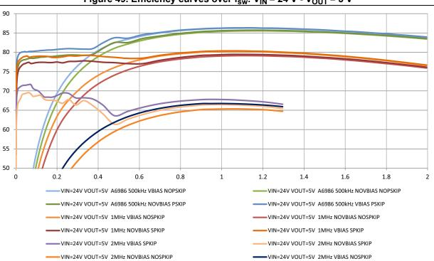
Figure 49. Efficiency curves over  $f_{sw}$ :  $V_{IN}$  = 24 V -  $V_{OUT}$  = 5 V
