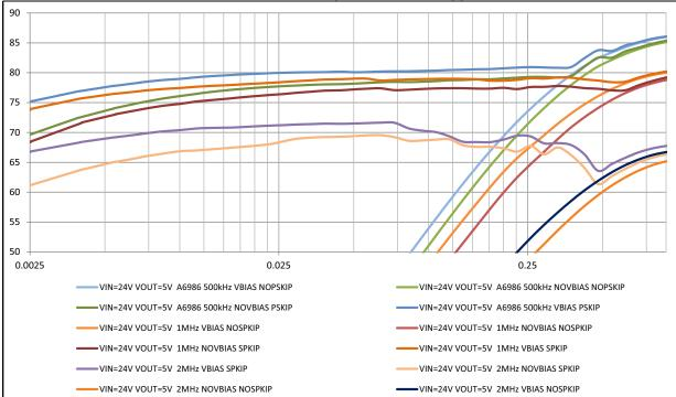
Figure 50. Efficiency curves over  $f_{sw}$ :  $V_{IN}$  = 24 V -  $V_{OUT}$  = 5 V (log scale)
