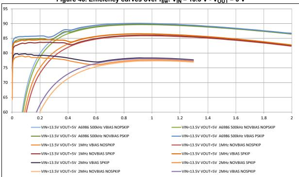
Figure 45. Efficiency curves over  $f_{sw}$ :  $V_{IN}$  = 13.5 V -  $V_{OUT}$  = 5 V
