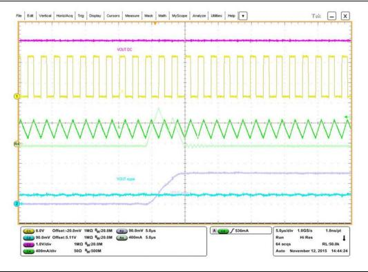
Figure 17. The regulator works in CCM
