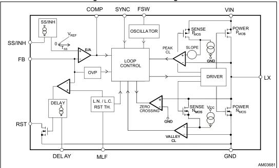
Figure 3. Internal block diagram
