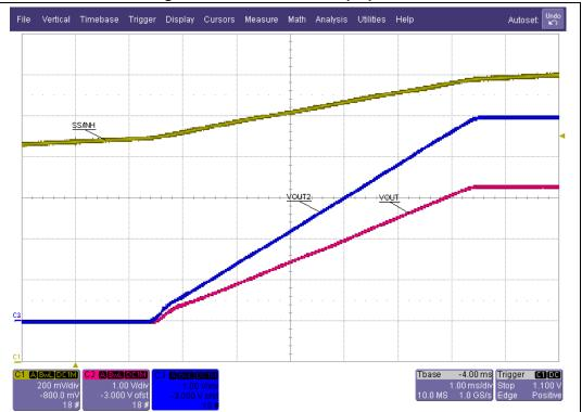
Figure 11. Ratiometric startup operation
