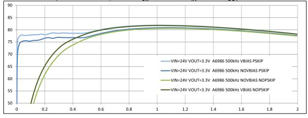
Figure 56. Efficiency curves:  $f_{sw}$  = 500 kHz -  $V_{IN}$  = 24 V -  $V_{OUT}$  = 3.3 V (log scale)
