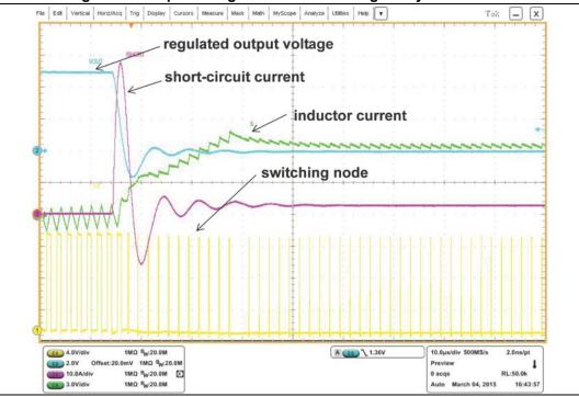
Figure 20. Output voltage oscillations during heavy short-circuit
