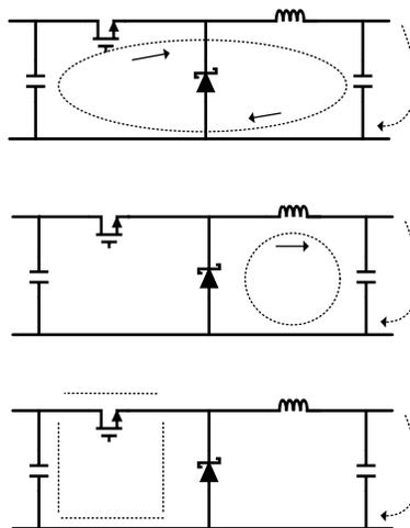
图 10-1. Current Flow in a Buck Application
