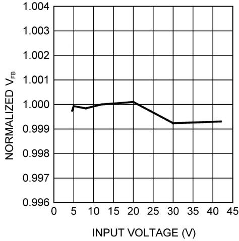
**图 6-7. Normalized Feedback Voltage vs Input Voltage**
