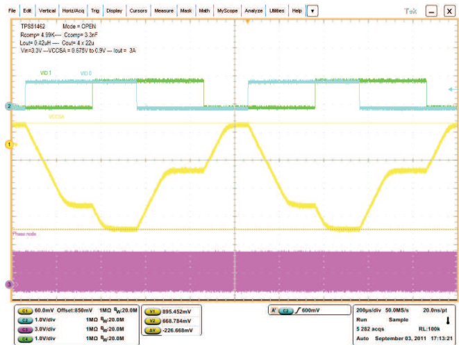
Figure 15. Mode=8, I_{OUT} = 3 A, VID Transitioning
