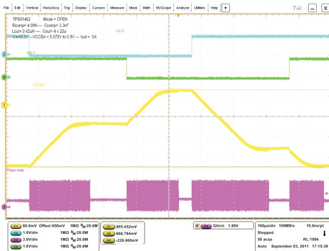
Figure 14. Mode=8, I_{OUT} = 0 A, VID Transitioning
