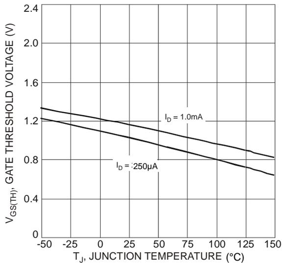
Fig. 9 Gate Threshold Voltage vs. Junction Temperature
