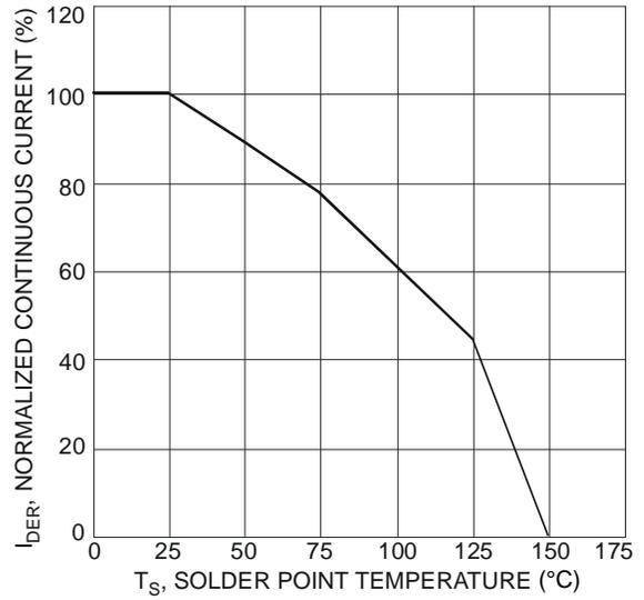
Fig 2. Normalized Continuous Current vs. Solder Point Temperature
