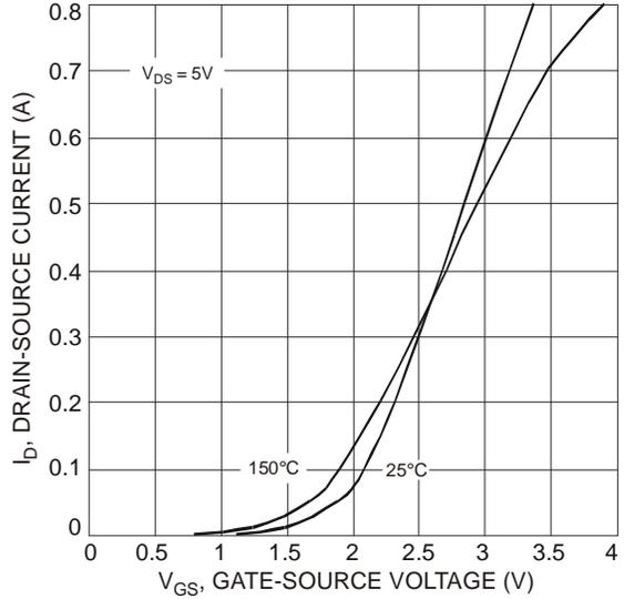
Fig. 6 Transfer Characteristics
