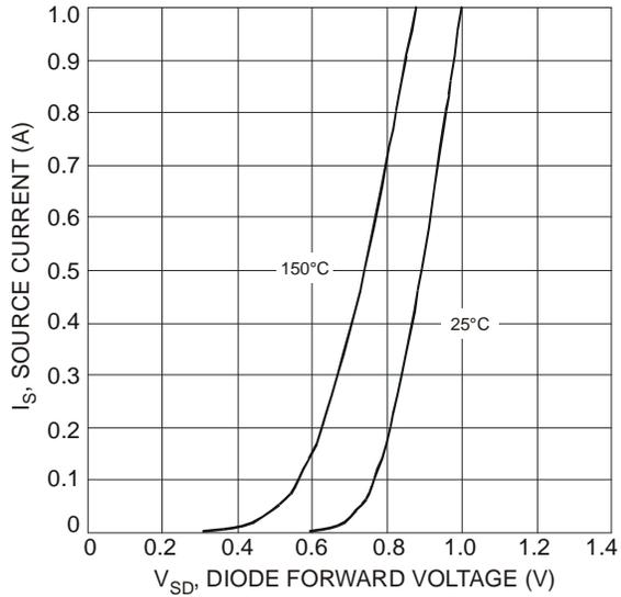
Fig. 13 Source Current vs. Diode Forward Voltage
