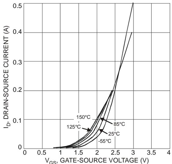
Fig. 10 Transfer Characteristics
