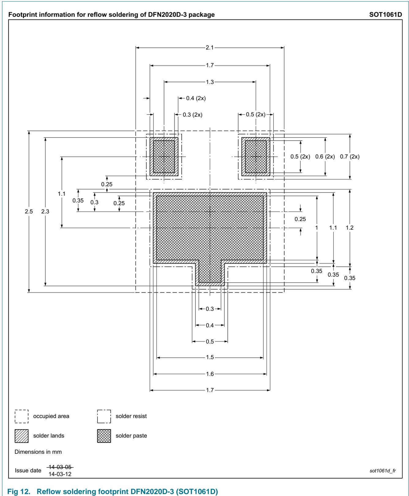
Fig 12. Reflow soldering footprint DFN2020D-3 (SOT1061D)
