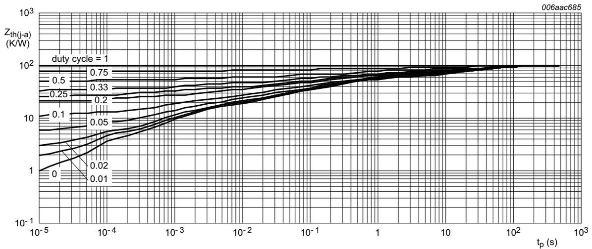
**Fig 4. Transient thermal impedance from junction to ambient as a function of pulse duration for; typical values**
