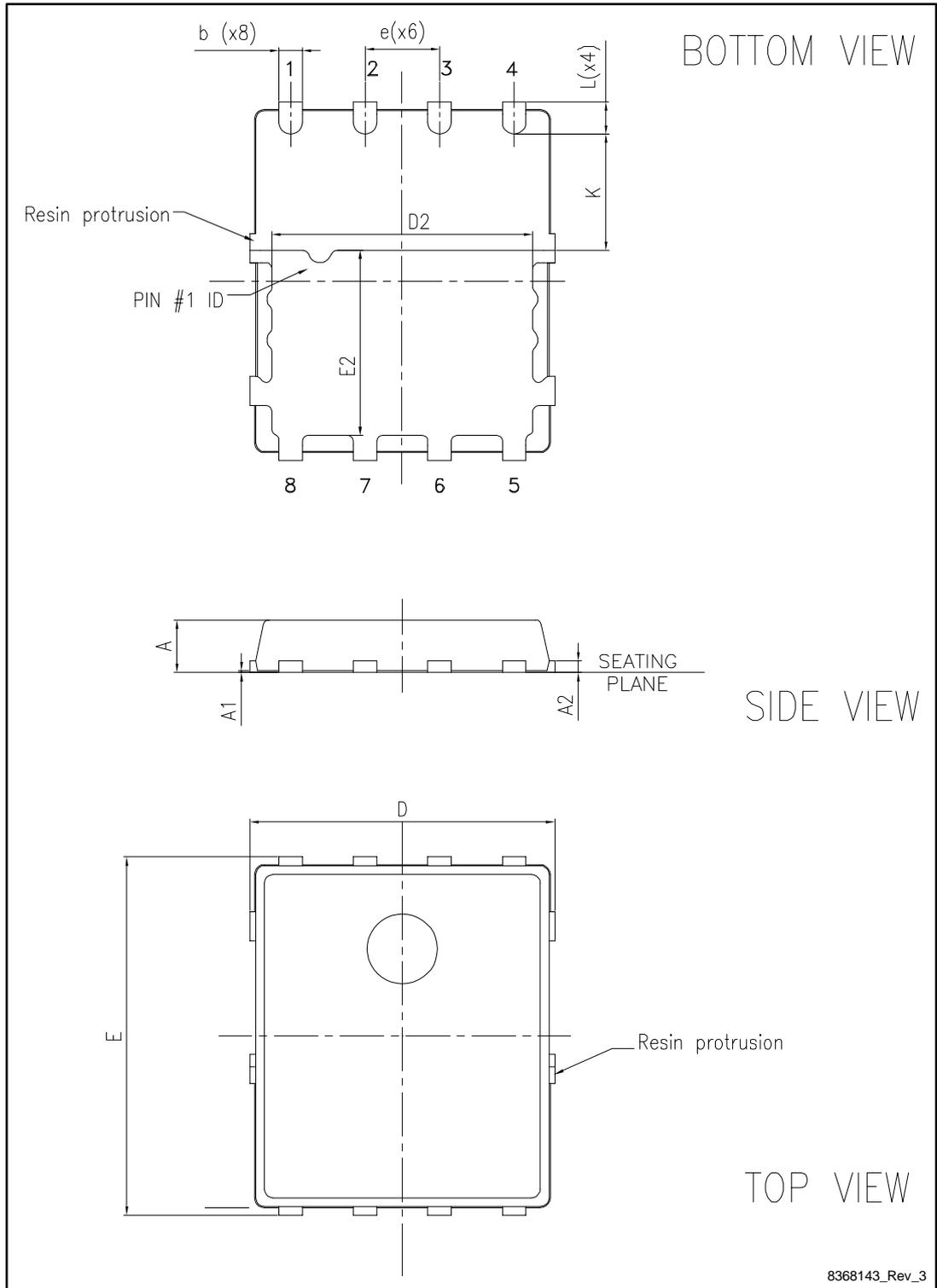
Table 9: PowerFLAT™ 5x6 HV mechanical data
