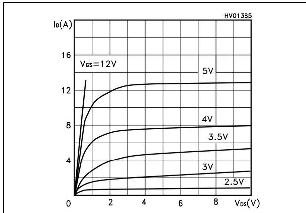
Figure 5. Transfer characteristics
