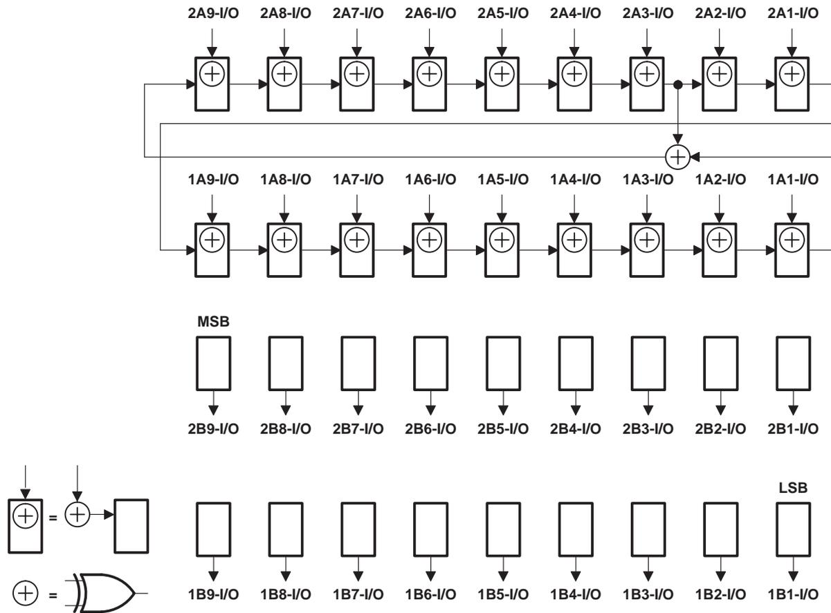
Figure 11. 18-Bit PSA/COUNT Configuration ( $\overline{1OEAB} = \overline{2OEAB} = 0$ ,  $\overline{1OEBA} = \overline{2OEBA} = 1$ )
