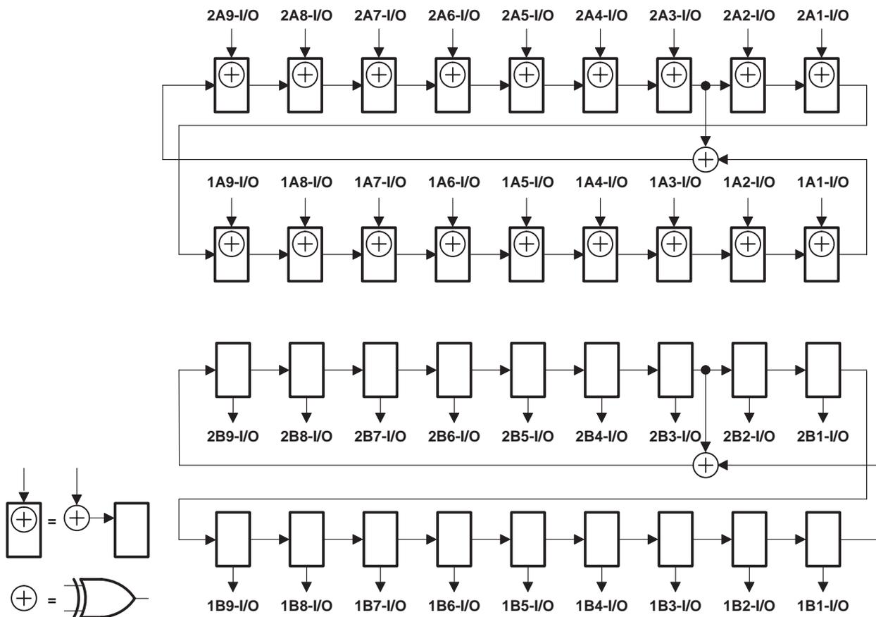
**Figure 9. 18-Bit PSA/PRPG Configuration ( $1\overline{0EAB} = 2\overline{0EAB} = 0$ ,  $1\overline{0EBA} = 2\overline{0EBA} = 1$ )**
