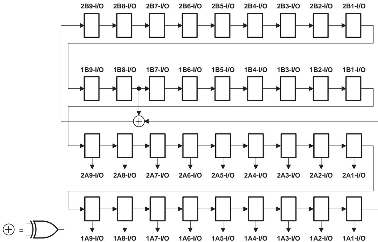
Figure 6. 36-Bit PRPG Configuration ( $1\overline{OEAB} = 2\overline{OEAB} = 1$ ,  $1\overline{OEBA} = 2\overline{OEBA} = 0$ )
