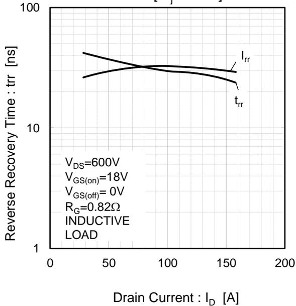
Fig.16 Recovery Characteristics vs. Drain Current [  $T_j=125^{\circ}\text{C}$  ]
