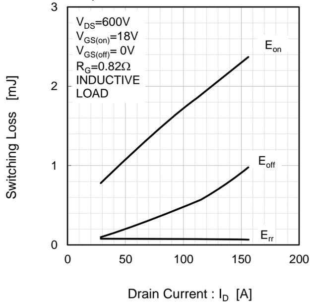
Fig.15 Recovery Characteristics vs. Drain Current [  $T_j=25^{\circ}\text{C}$  ]
