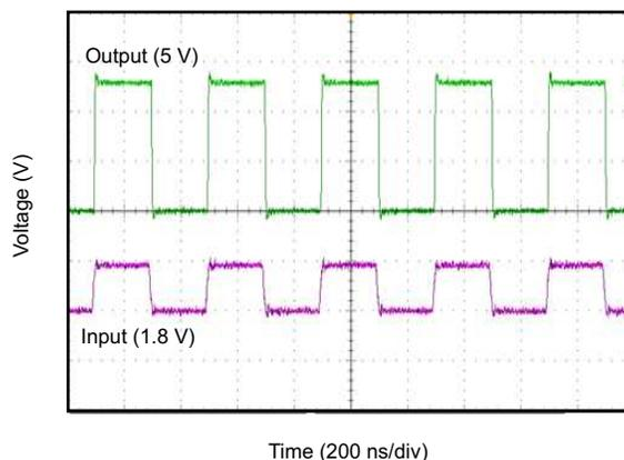
**Figure 6. Translation Up (1.8 V to 5 V) at 2.5 MHz**
