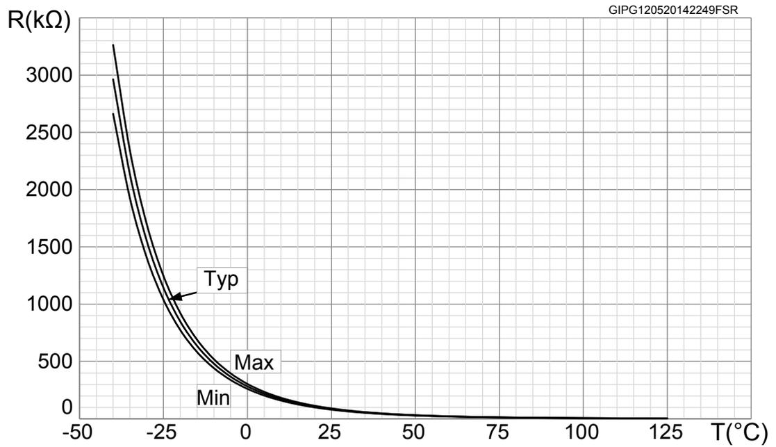
Figure 9. NTC resistance vs temperature - zoom
