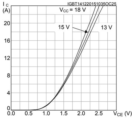
Figure 12.  $V_{CE(sat)}$  vs collector current
