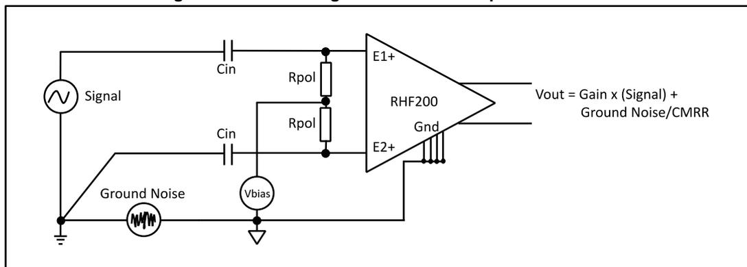
Figure 51: Incorrect single-to-differential implementation
