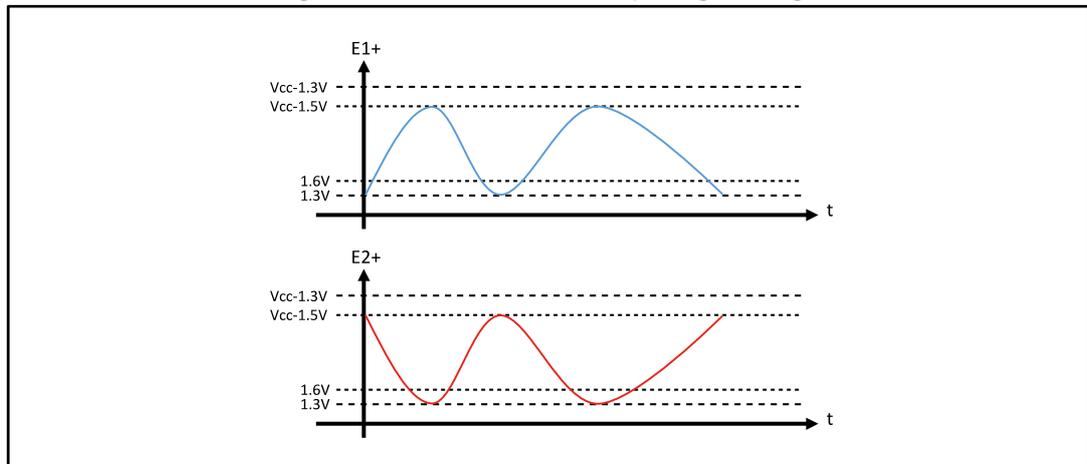
Figure 47: Second correct use of the input signal range
