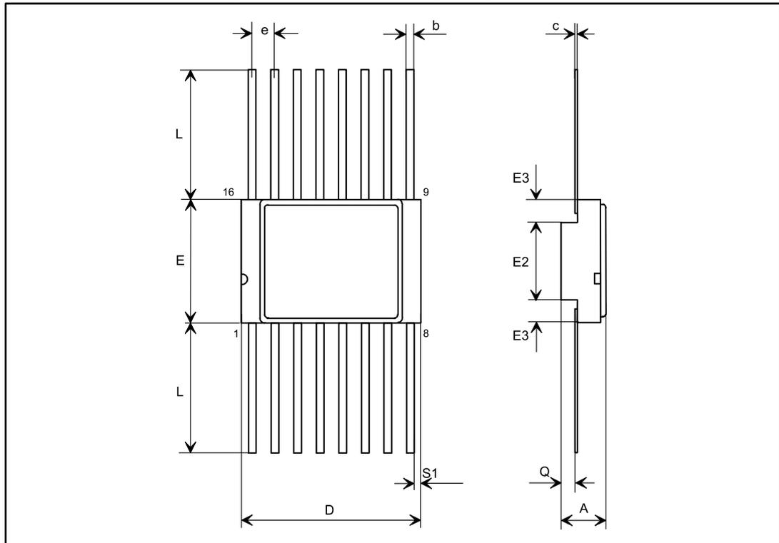
1. The upper metallic lid is electrically connected to pin16.
