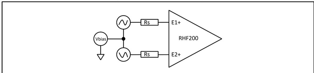
Figure 45: AC input coupling
