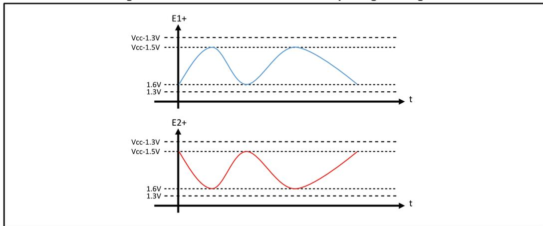
Figure 48: Incorrect use of the input signal range
