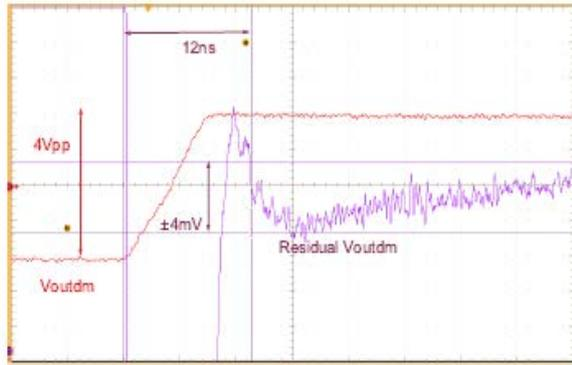
$4.5\text{V} \leq V_{cc} \leq 5.5\text{V}$ ,  $A_v = 2$ ,  $R_L = 200\Omega$ ,  $5\text{ns/div}$ ,  $T_a = -55^\circ\text{C}$
