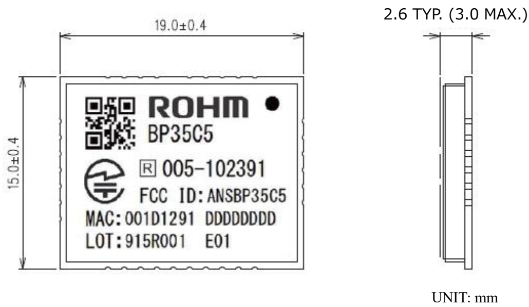
Fig. 3. Outline Dimensions Diagram
