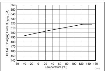
Figure 6-28. I<sub>CHG</sub> DESAT Charging Current vs. Temperature
