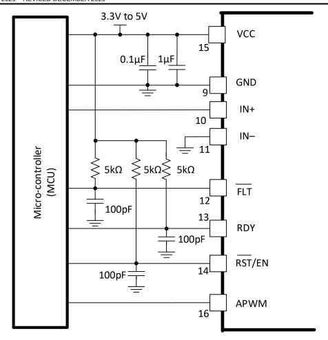
Figure 9-3. FLT, RDY and RST/EN Pins Circuitry
