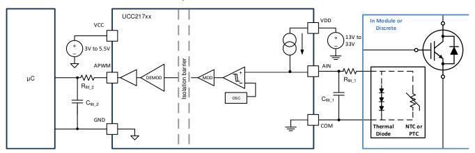
Figure 9-8. APWM Channel with Filtered Output
