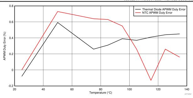
Figure 9-11. APWM Duty Error with Single-Point Calibration
