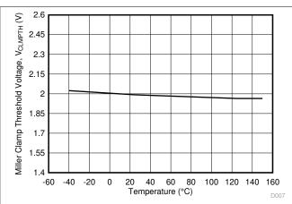
Figure 6-20. V<sub>CLMPTH</sub> Miller Clamp Threshold Voltage vs. Temperature
