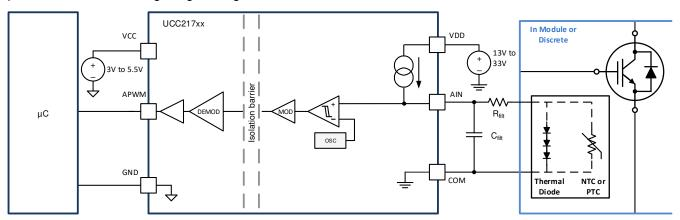
Figure 8-7. Isolated Analog to PWM Signal
