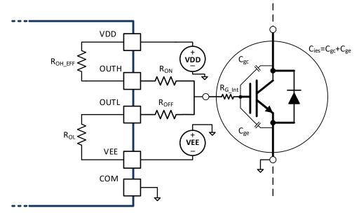
Figure 9-5. Output Model for Calculating Peak Gate Current
