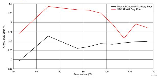
Figure 9-10. APWM Duty Error Without Calibration
