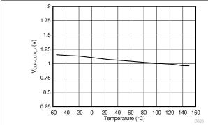
Figure 6-19. V<sub>CLP-OUT(L)</sub> Short Circuit Clamping Voltage vs. Temperature
