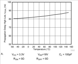
Figure 6-14. Propagation Delay t<sub>PDHL</sub> vs. Temperature
