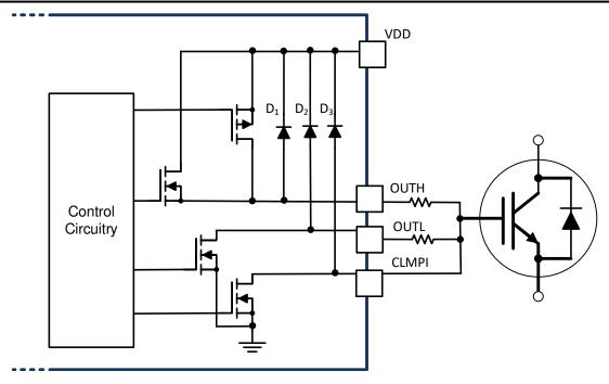
Figure 8-3. Short Circuit Clamping
