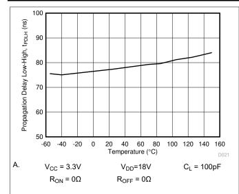
Figure 6-13. Propagation Delay t<sub>PDLH</sub> vs. Temperature
