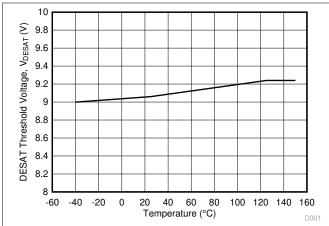
Figure 6-23. V<sub>DESAT</sub> DESAT Threshold Voltage vs. Temperature
