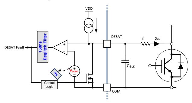
Figure 8-5. DESAT Protection
