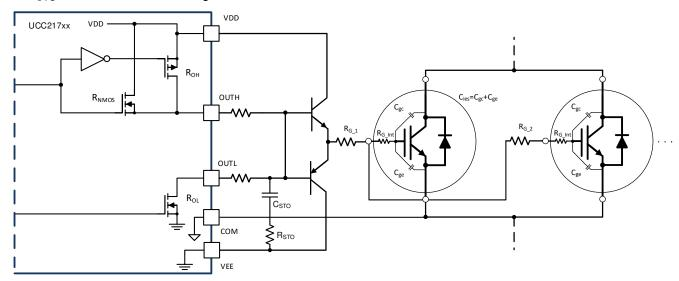
Figure 9-13. Current Buffer for Increased Drive Strength
