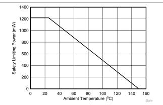
Figure 6-2. Thermal Derating Curve for Limiting Power per VDE
