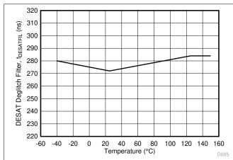
Figure 6-27. t<sub>DESATFIL</sub> DESAT Deglitch Filter vs. Temperature
