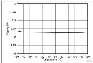
Figure 6-17. V<sub>OUTPD</sub> Output Active Pulldown Voltage vs. Temperature
