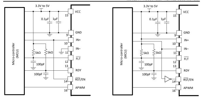
Figure 9-4. Automatic Reset Control
