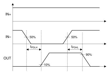
Figure 7-2. Inverting Logic Propagation Delay Measurement
