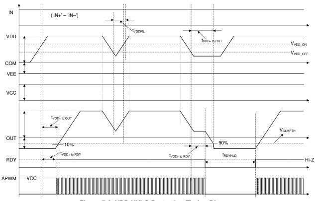
Figure 7-9. VDD UVLO Protection Timing Diagram
