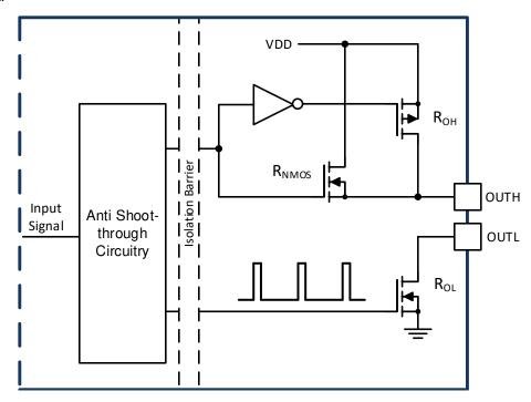
Figure 8-1. Gate Driver Output Stage
