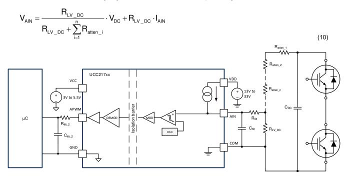
Figure 9-12. DC-link Voltage Sensing Configuration
