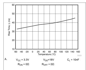
Figure 6-15. t<sub>r</sub> Rise Time vs. Temperature
