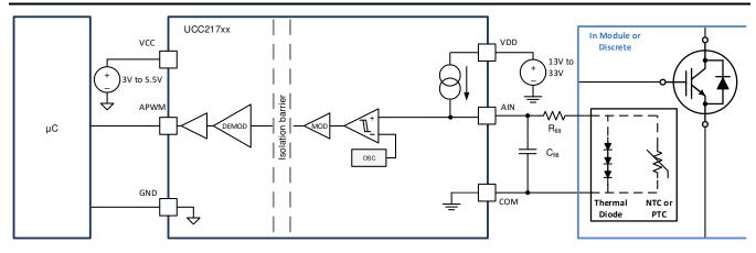
Figure 9-7. Thermal Diode or Thermistor Temperature Sensing Configuration
