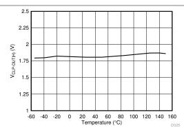
Figure 6-18. V<sub>CLP-OUT(H)</sub> Short Circuit Clamping Voltage vs. Temperature
