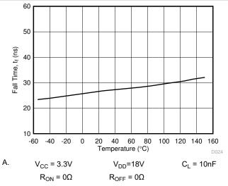
Figure 6-16. t<sub>f</sub> Fall Time vs. Temperature
