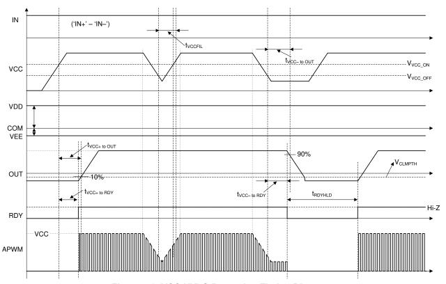
Figure 7-8. VCC UVLO Protection Timing Diagram
