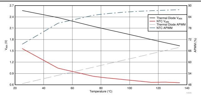
Figure 9-9. Thermal diode and NTC V<sub>AIN</sub> and Corresponding Duty Cycle at APWM
