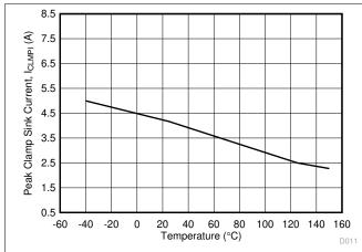
Figure 6-21. I<sub>CLMPI</sub> Miller Clamp Sink Current vs. Temperature
