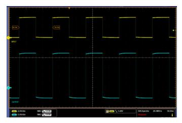
Figure 9-14. PWM input (yellow) and driver output (blue)
