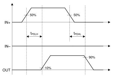
Figure 7-1. Non-inverting Logic Propagation Delay Measurement
