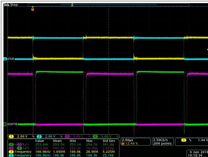
图 42. Bench Test Waveform for INA/B and OUTA/B
