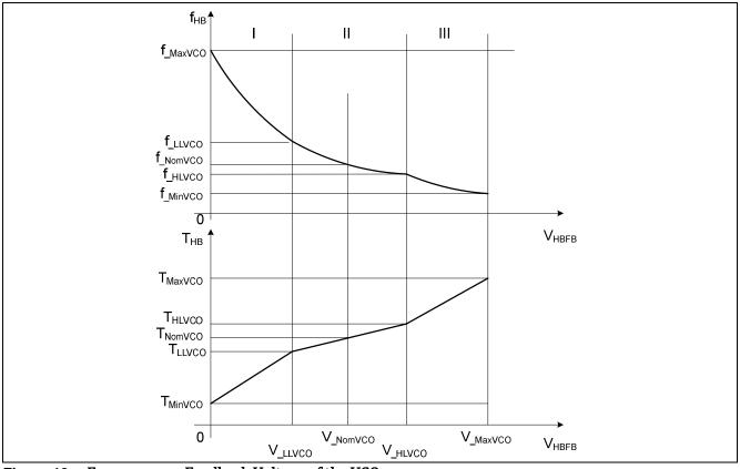
Figure 13Frequency vs. Feedback Voltage of the VCO
