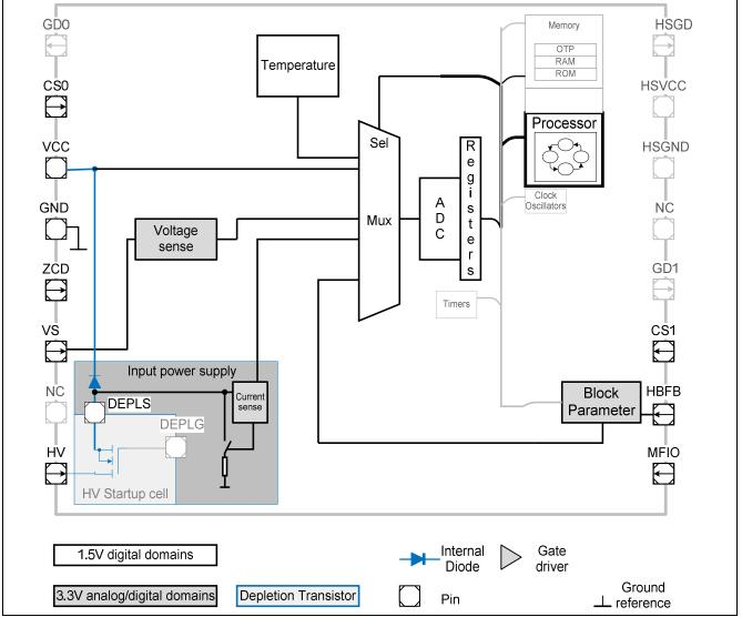
Figure 6 Voltage and current sensing multiplexing to ADC
