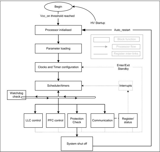
Figure 5 Overview of Processor operations
