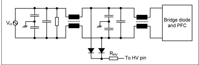
Figure 9 Circuit with AC detection with EMI filter
