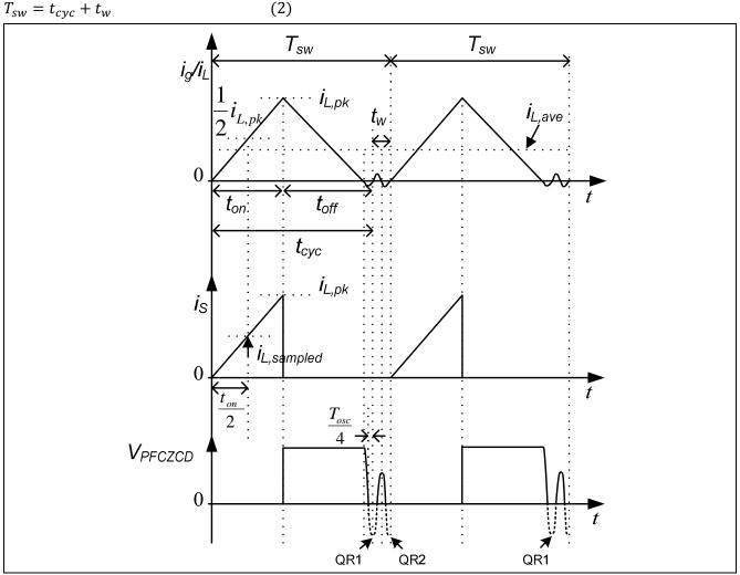
Figure 11 Current and timing in QR2 Operation
