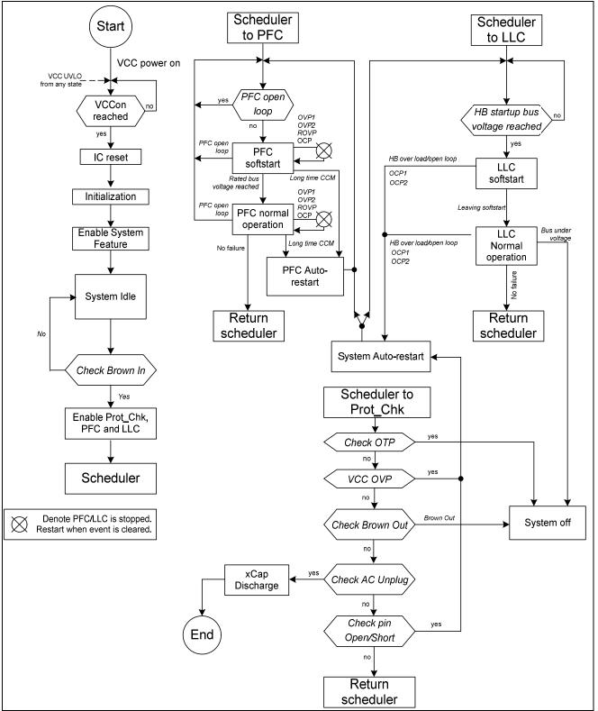
Figure 14 General Operation Flow of the Controller
