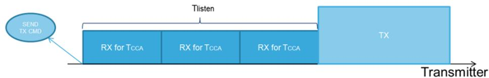
If the channel is busy and persistent\_mode bit is 1, the device checks the channel continuously in  $T_{cca}$  periods. When the channel becomes free, it must assert channel free for a number of **NUM\_OF\_CCA\_PERIOD** ( $T_{listen}$ ) before transmitting:
