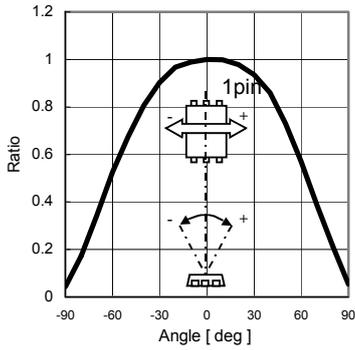
Fig.4 Directional Characteristics 1
