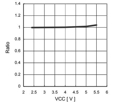
Fig.9 IOUT VCC dependency
