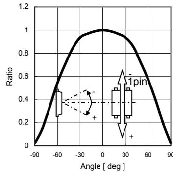
Fig.5 Directional Characteristics 2
