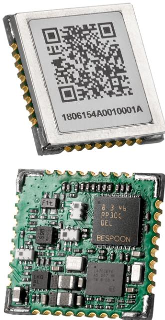
*B-UWB-MOD1 with (top view) and without (bottom view) cover cap. Pictures are not contractual.*
