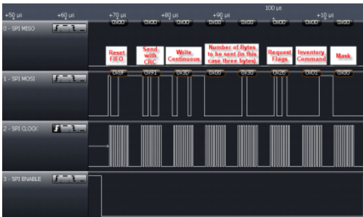
Figure 6-22. Inventory Command Sent From MCU to TRF7964A
