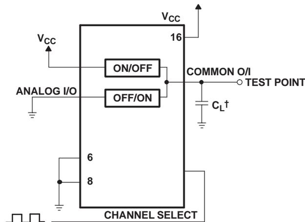
† Includes all probe and jig capacitance
