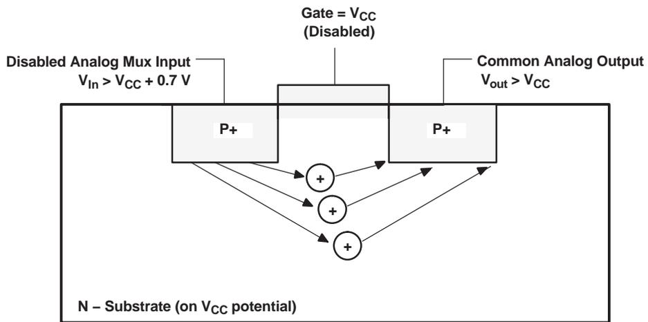
**Figure 4. Diagram of Bipolar Coupling Mechanism**
