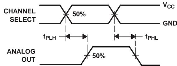
**Figure 9. Propagation Delays, Channel Select to Analog Out**
