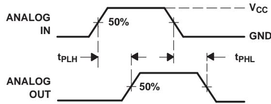
Figure 11. Propagation Delays, Analog In to Analog Out
