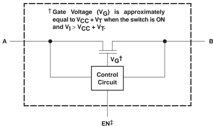
† EN is the internal enable signal applied to the switch.
