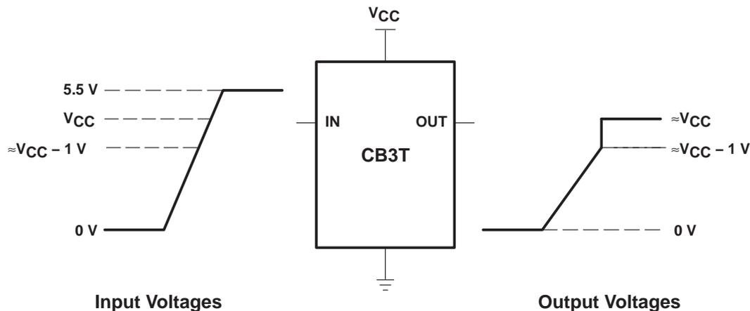
NOTE A: If the input high voltage ( $V_{IH}$ ) level is greater than or equal to  $V_{CC} - 1\text{ V}$ , and less than or equal to 5.5 V, then the output high voltage ( $V_{OH}$ ) level will be equal to approximately the  $V_{CC}$  voltage level.
