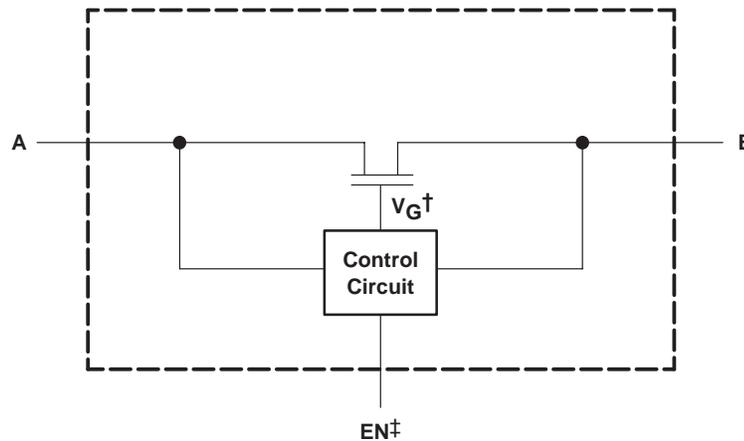
† Gate Voltage ( $V_G$ ) is approximately equal to  $V_{CC} + V_T$  when the switch is ON and  $V_I > V_{CC} + V_T$ .
